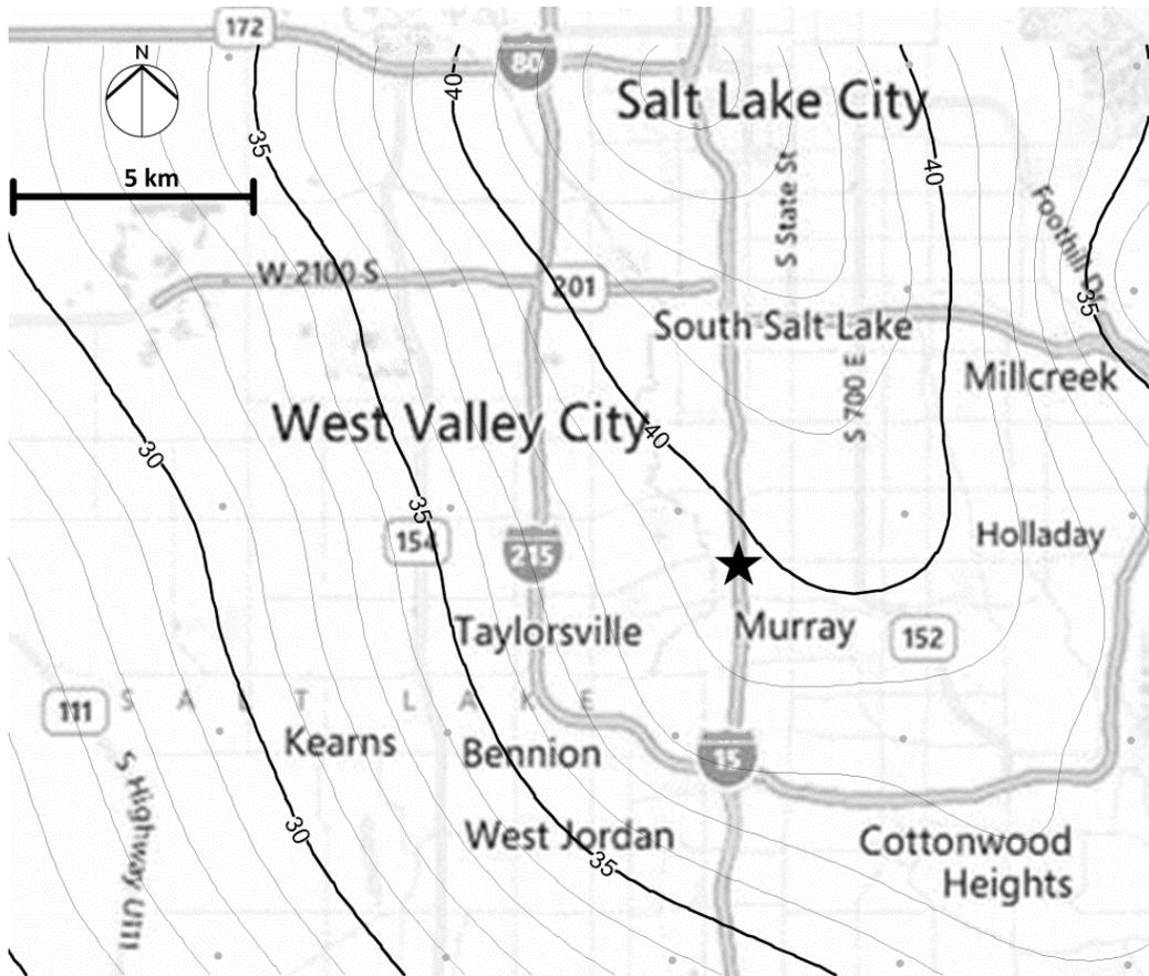
**Figure 3-3.** Liquefaction loading map ( $T_R = 1,033$  years) showing contours of  $CSR^{ref}(\%)$  for a portion of the Salt Lake Valley in Utah (after Ulmer 2015)
